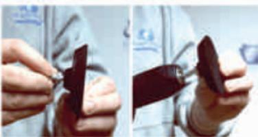
**Warning!** The metal polishing compound is an abrasive compound, please make sure the surface you are working on is not plated or coated as this compound can remove it.
